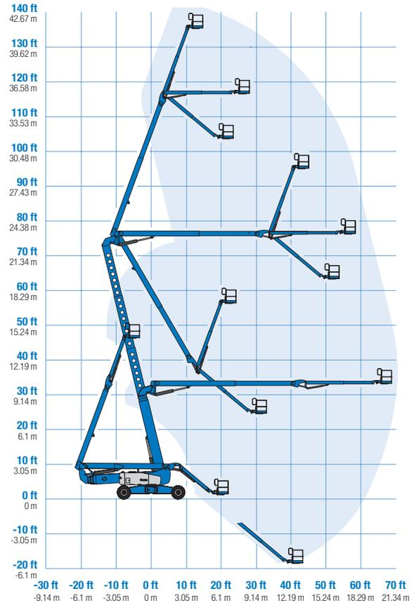
\* The metric equivalent of working height adds 2 m to platform height. U.S. adds 6 ft to platform height.
